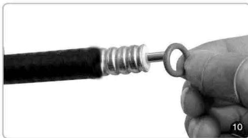
Chamfer inner conductor 1 \times 45^\circ with flat file.
