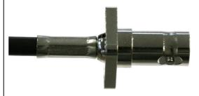
**8.** Crimp the crimp sleeve with a crimp tool; herewith the copper braid will be clamped between the socket housing and the crimp sleeve.
