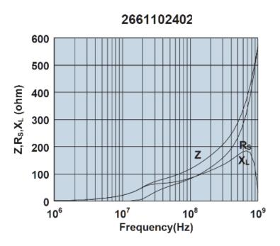
Impedance, reactance, and resistance vs. frequency.
