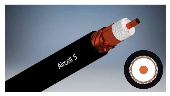
Aircell 5 is a flexible and thin coaxial cable with 5 mm outer diameter for the frequency range from DC to 10 GHz. Its low loss characteristics in relation to the diameter and the ability to use standard RG 58 connectors make this cable the number one choice not only for Wireless LAN applications but also for general RF communications.
