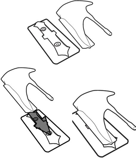
Carefully clean the area before to stick the adhesive and wait 24 hours before submersion for best adhesion.
