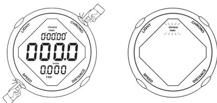
**To enter in the programming mode, you have to be either in MANUAL chronometer mode with stopped countdown timer or in automatic and not read the signal.**
