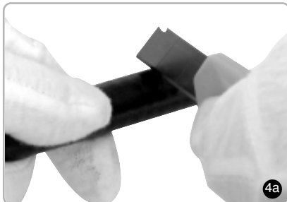
Strip off some cable jacket (20-26mm).
