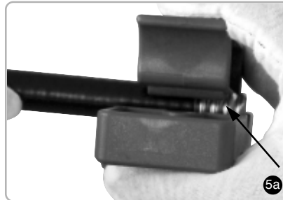
Place the manual cutting tool so that blade cuts second corrugation from top.
