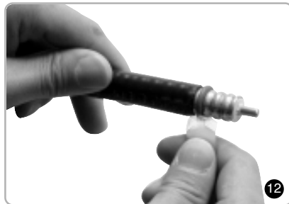
Lubricate O-ring with grease.
