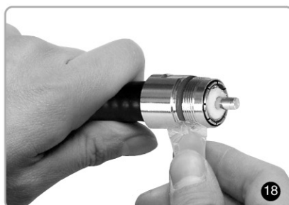
Lubricate O-ring which is on connector back part.
