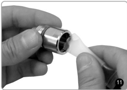
Lubricate inner O-ring.
